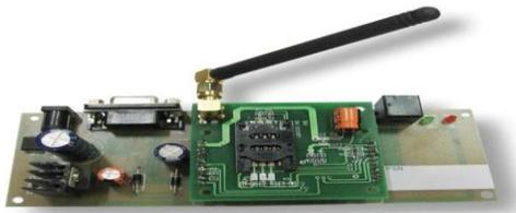
Fig 2: GSM modem GPS RECEIVER
