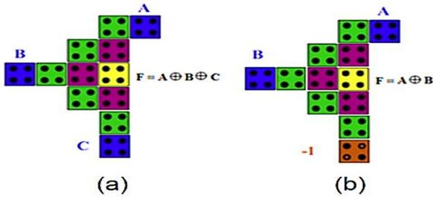
**Fig 6:** The layout of proposed XOR gate in [24], (a) 3-input XOR, (b) 2-input XOR.
