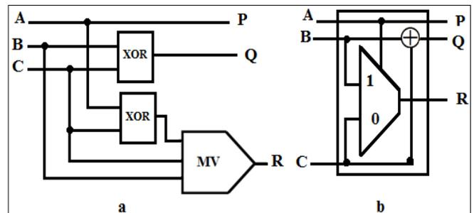
Fig 4: The proposed reversible gate (a) schematic and (b) symbol
