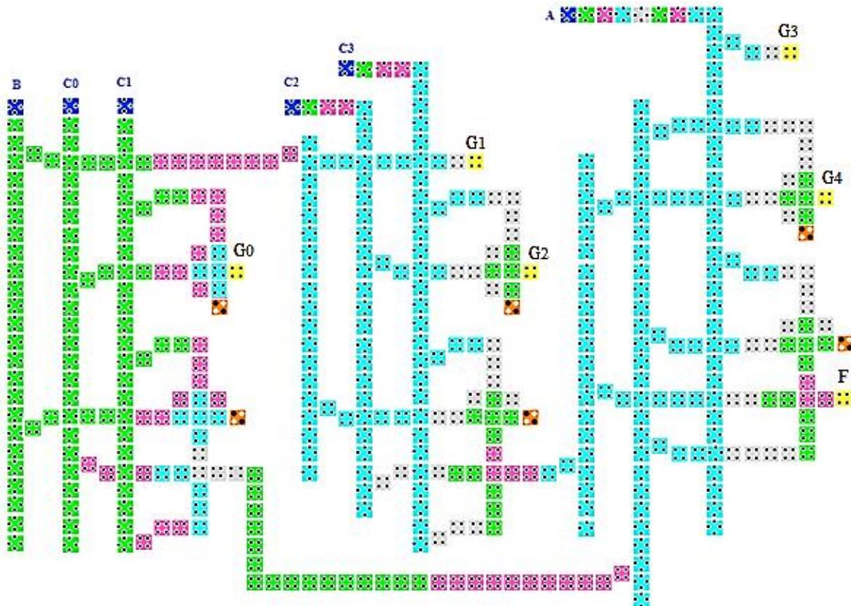
Fig 15: The QCA layout of the proposed RLU
