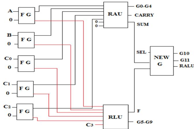
Fig 11: Schematic diagram of the proposed reversible ALU
