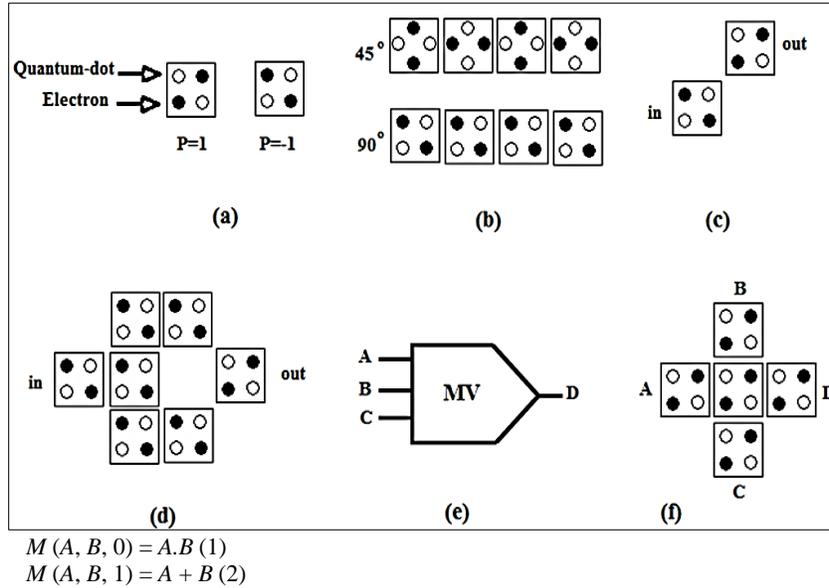
**Fig 1:** Basic QCA structures. (a) QCA cell, (b) binary wire ( $90^\circ$ ) and inverter chain ( $45^\circ$ ), (c, d) inverter gate, (e) a Schematic view and (f) b QCA design of Three-input majority gate.
