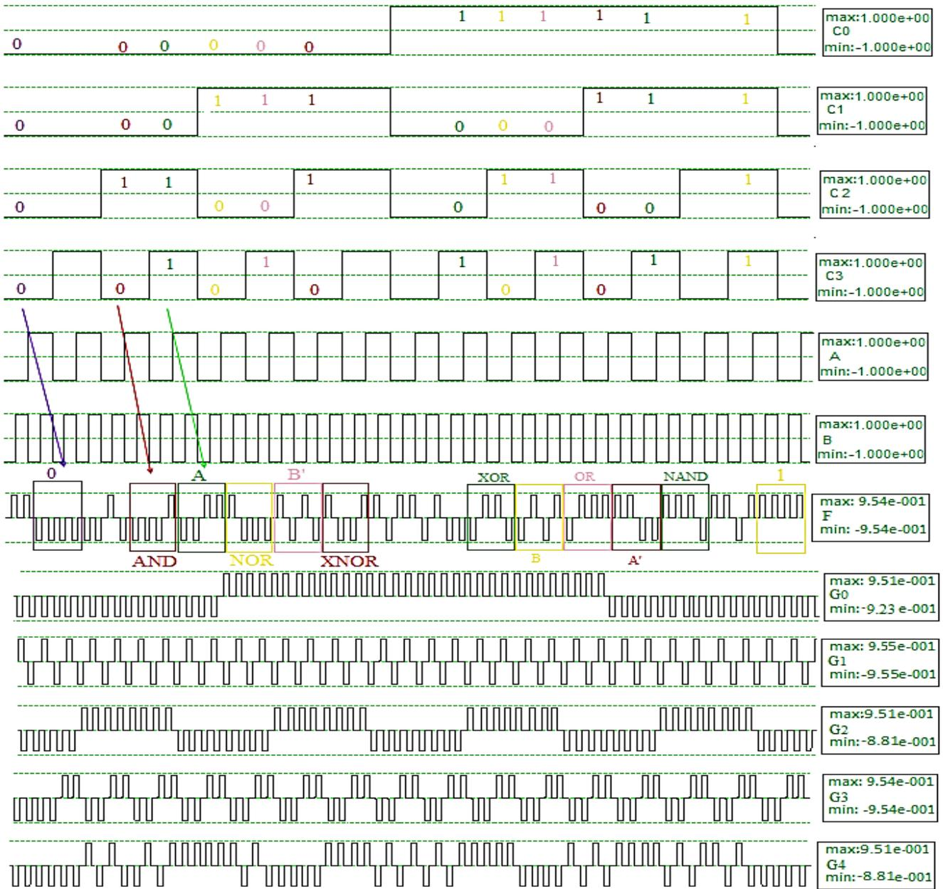
Fig 18: The simulation results of the proposed RLU.
