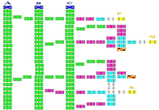
**Fig 7:** The QCA layout of proposed reversible gate
