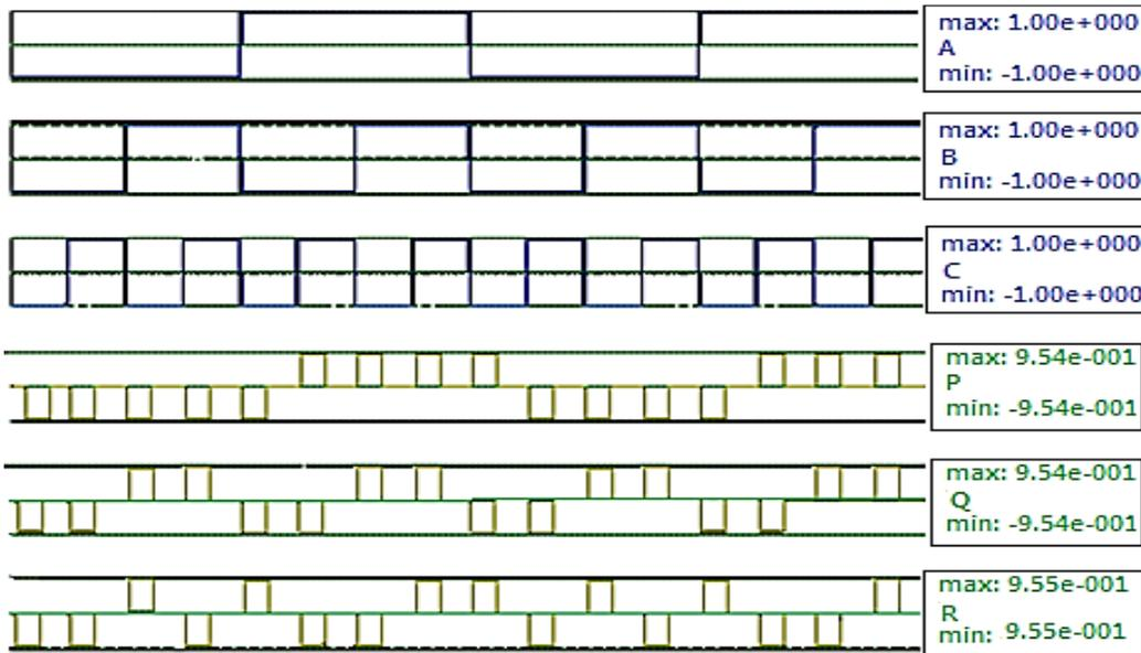
**Fig 8:** The simulation result of the proposed reversible gate
