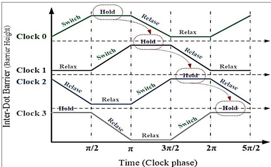
**Fig 2:** QCA clocking with four phases.
