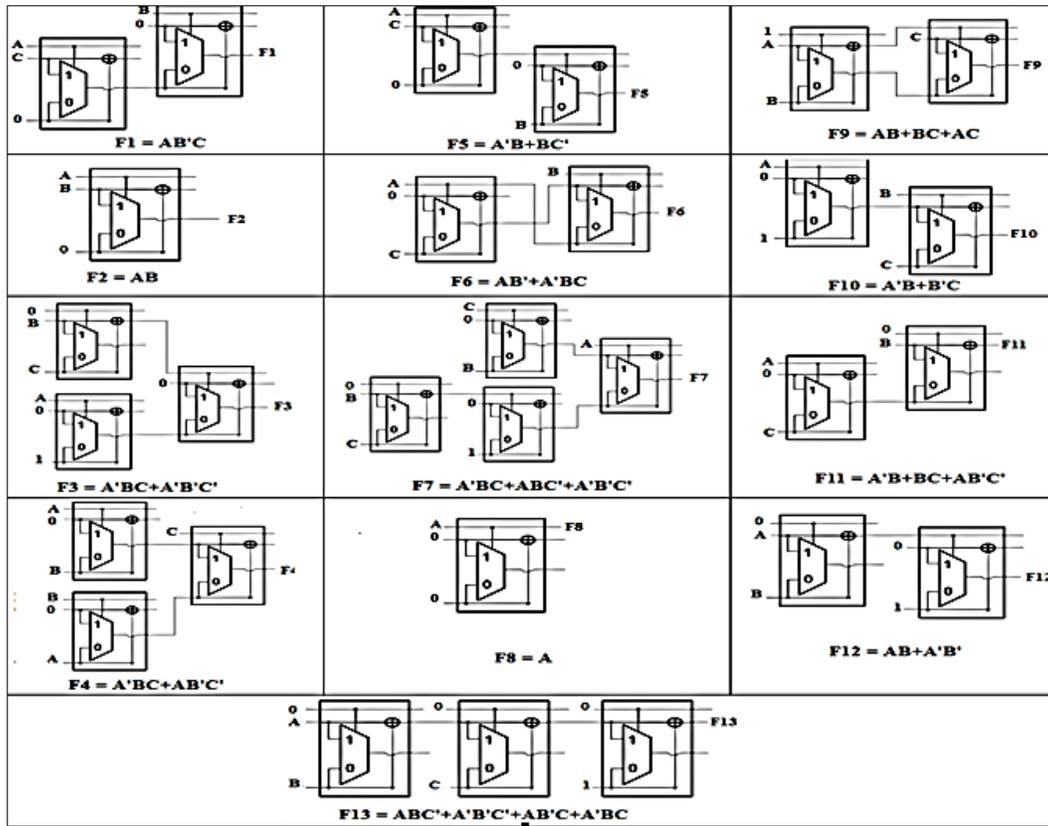
**Fig 5:** Reversible implementation of the 13 standard functions
