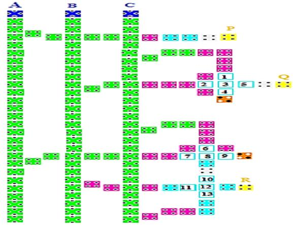
**Fig 9:** The layout of possibility missing cells of the proposed gate
