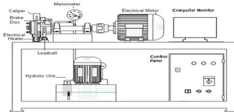
**Fig 1:** The brake lining test device <sup>[9]</sup>
