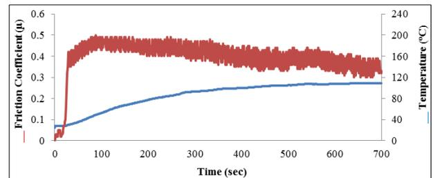
**Fig 3:** Friction coefficient-temperature-time graph of 6% nano borax sample
