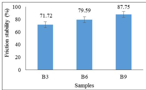
Fig 5: Friction stability of pad samples (%)
