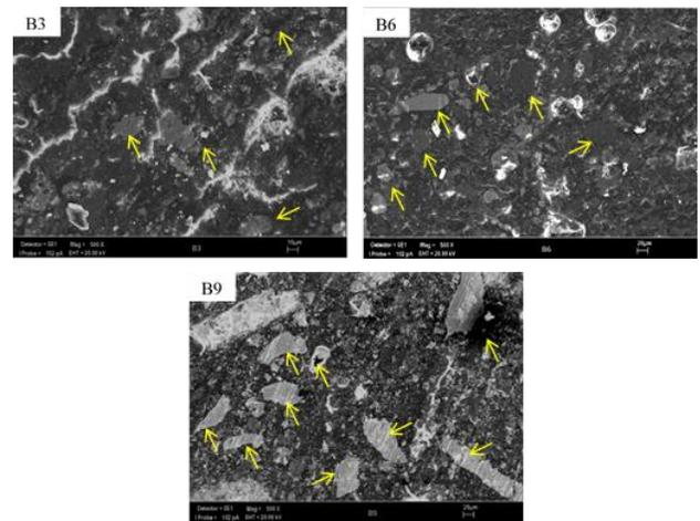
Fig 6: SEM morphologies of frictional surface of pad samples
