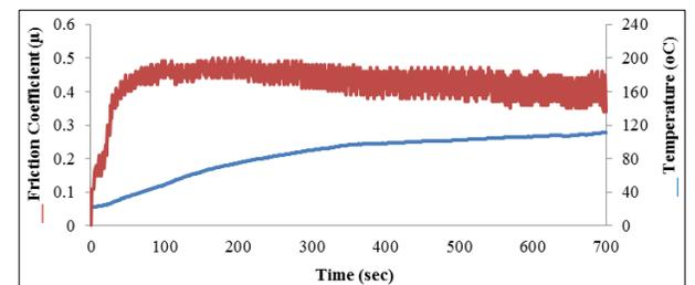
**Fig 4:** Friction coefficient-temperature-time graph of 9% nano borax sample
