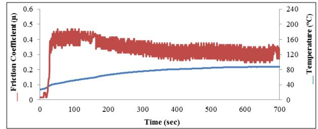
**Fig 2:** Friction coefficient-temperature-time graph of 3% nano borax brake pad sample
