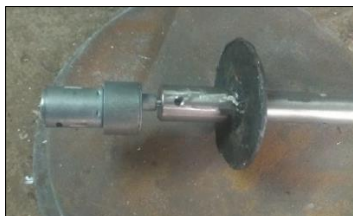
Fig 7: Spindle with limiting disc
