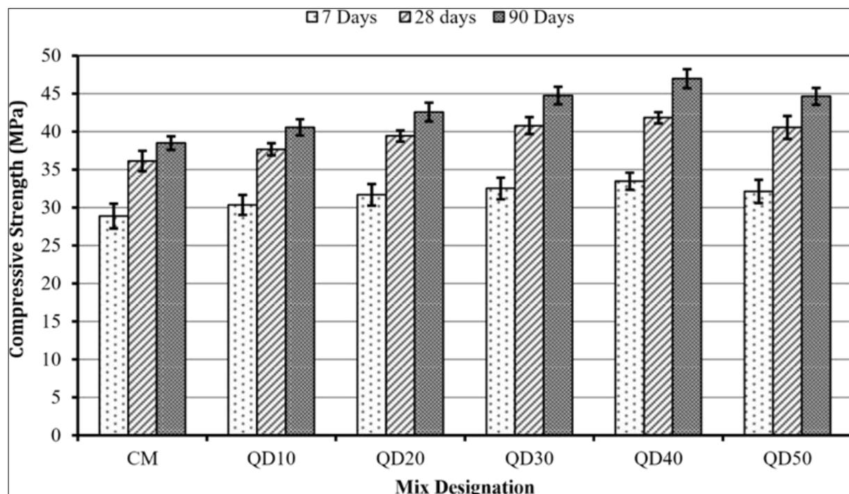
**Fig 5:** Effect of Replacement of Natural Sand with Crushed sand on Compressive Strength of Concrete
