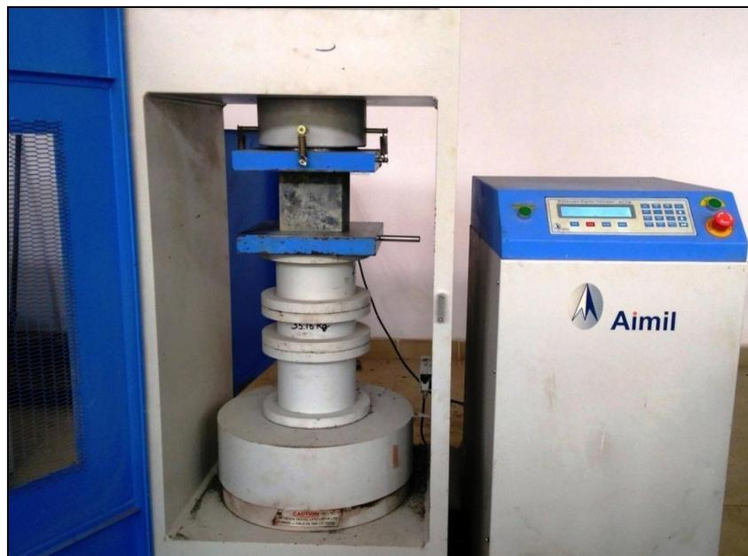
**Fig 2:** Compressive Strength Test on Compression Testing Machine
