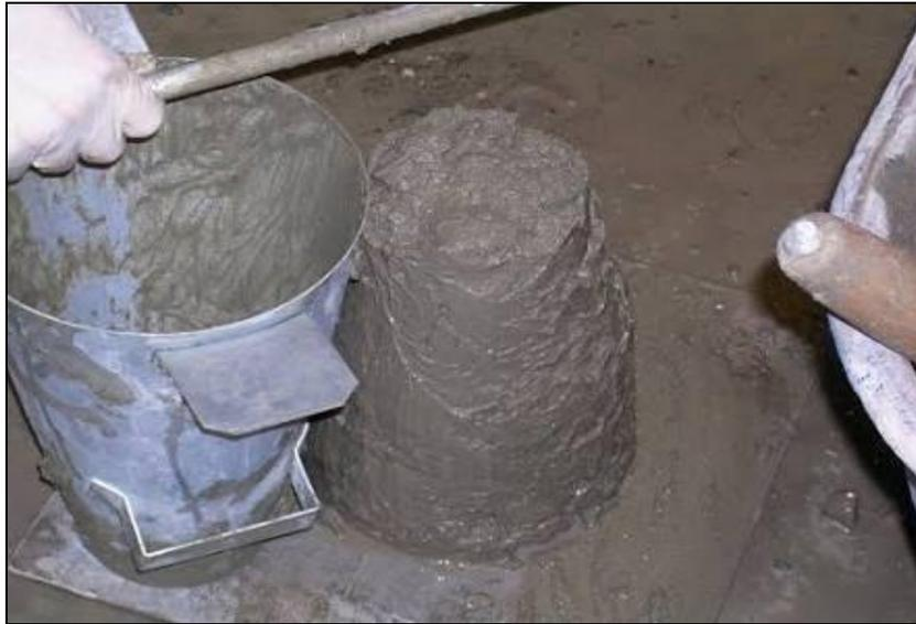
**Fig 1:** Slump Test of Concrete
