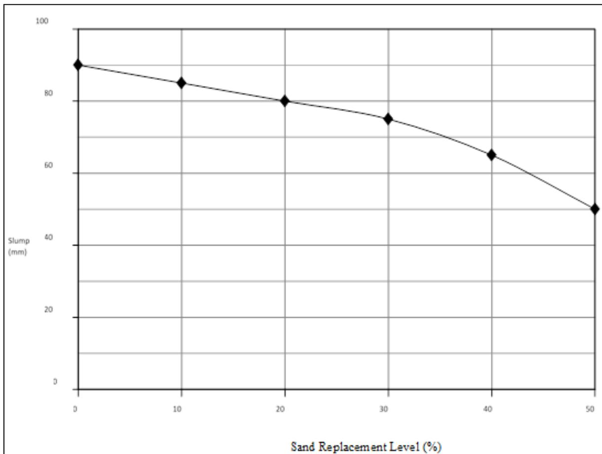
**Fig 4:** Effect of Replacement of Natural Sand with Crushed sand on Workability of Concrete
