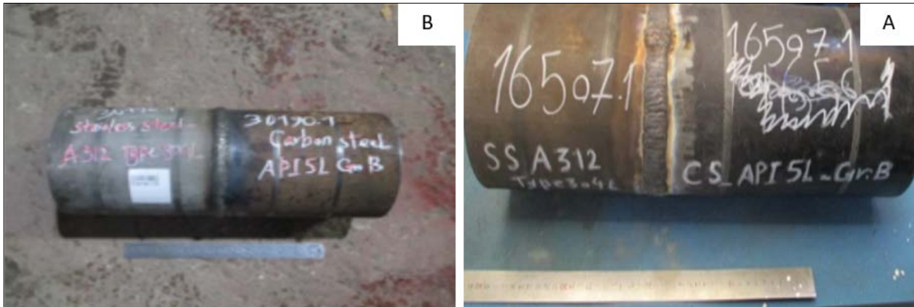
Fig 9: Welded Joint between Stainless Steel and Carbon Steel ((A) Close-up view of the welded joint between stainless steel (SS A312) and carbon steel (CS API 5L Gr. B), showing the weld seam and markings. (B) Full view of the welded specimen, highlighting material specifications and dimensions.
