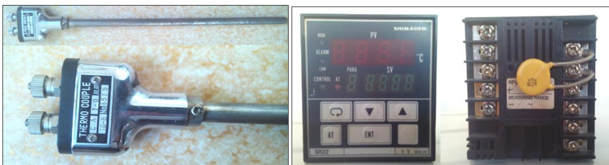
Fi 9g 3: Thermocouple and digital temperature controller used for measurement.
