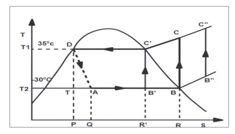
Each segment of the cycle-compression, heat rejection, expansion, and heat absorption-has a distinct thermodynamic behaviour. Notably, during the heat rejection phase, a portion of the refrigerant becomes superheated, sometimes reaching temperatures 30-40°C above the saturation point. This superheat represents a valuable opportunity for energy recovery.
