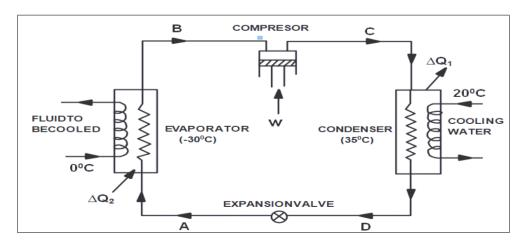
In this cycle, the refrigerant undergoes several transformations. Initially, low-pressure, low-temperature vapour is compressed into a high-pressure, high-temperature state. This vapour
