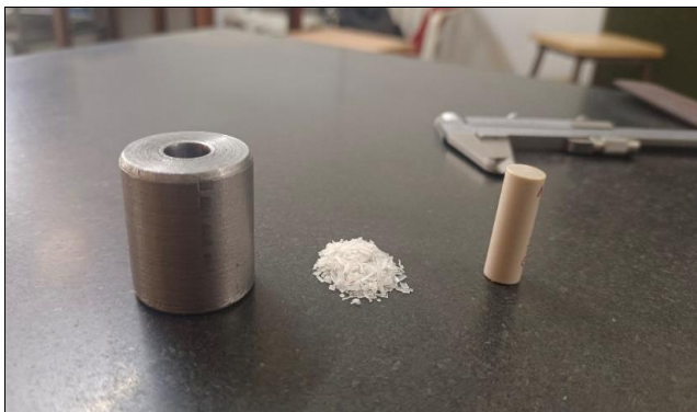
Fig 2: MS Mold, UHMWPE granules and PEEK pin.
