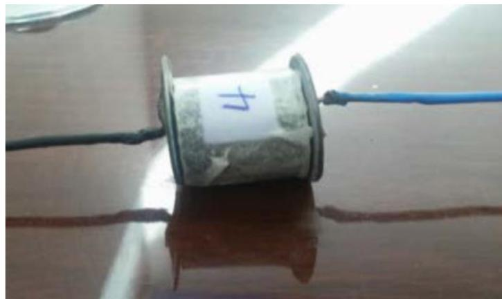
Fig 6: Insulators specimen under test
