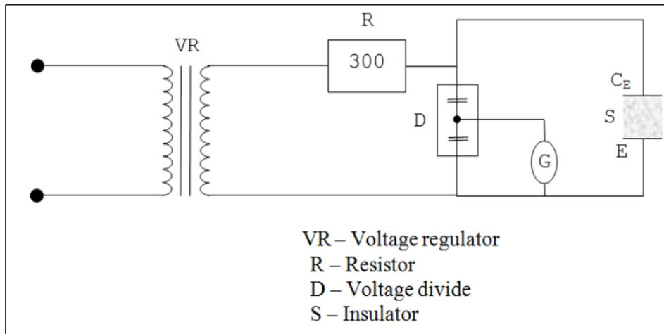
Fig 1: Test Circuit
