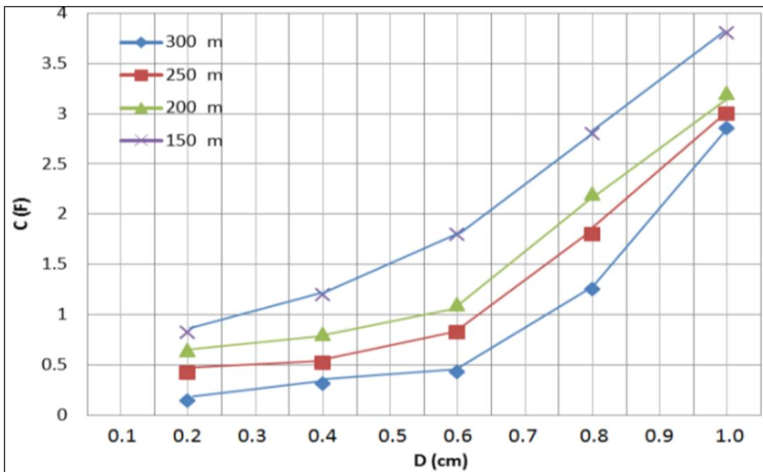
Fig 4: Capacitance of insulator over the length of insulator
