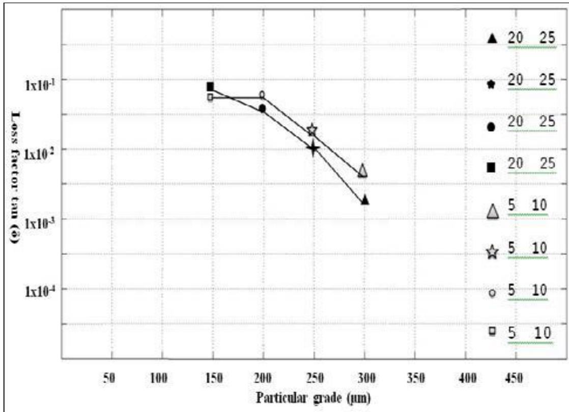
Fig 5: Relation between particles grade and tan δ at constant percent of cement and resin at: 270 volte, 50 Hz, Portland – cement 20%, Resin 25%
