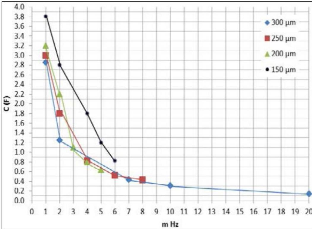
Fig 3: Capacitance of insulator over the frequency
